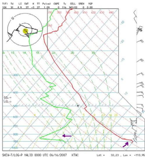
Figure 6 - Skew-T plot of TUS sounding for 0000 UTC June 16, 2007. A very dry layer is present again above the surface. The temperature structure on the roof top, and just above, seems very strange (sounding from UCAR RAP upper-air page).
