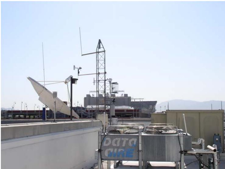
Figure 4 - Photo of the new surface observing system installed on the roof of the NWS/USGS building looking east toward the U of A football stadium.
