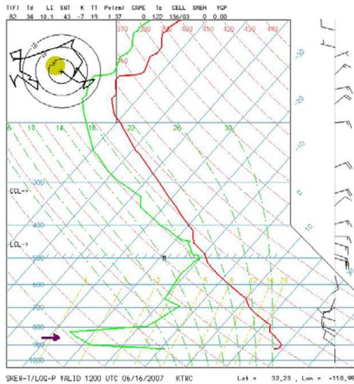
Figure 5 - Skew-T plot of TUS sounding for 1200 UTC June 16, 2007. Note that the very dry layer indicated by the purple arrow is due to hygrometer problems of the Sippican sonde (sounding from UCAR RAP upper-air page).
