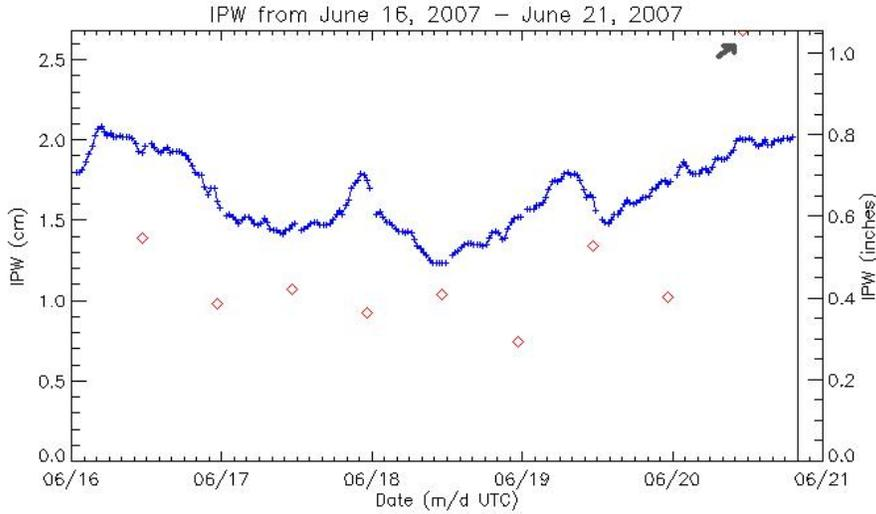
Figure 7 - Time series of integrated precipitable water (IPW) from GPS data (blue) for TUS from June 16 through June 21, 2007. The RRS sonde flights' IPW (red diamonds) for the same period are shown. For this period the RRS sonde data are consistently dry relative to the GPS IPW (both morning and evening flights) except that the morning flight on the 20th was strangely too moist (arrow indicates that diamond, which is almost off the figure - figure from NOAA FSL).
